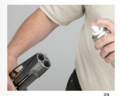
clean the barrel first with the tubes installed and then remove and clean the tubes themselves as described before. Make sure, that after cleaning, no solvent is left in the gun. Cleaning solvent must be removed entirely. For gun storage, apply a very thin film of gun pro or any other high quality gun oil into chamber and bore for corrosion protection.
