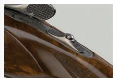
and simultaneously sliding the safety switch to the rear to put the gun "on safe". The gun is taken "off safe" and made ready to fire by depressing the button and sliding the safety switch forward. When the gun is "on safe", the letter "S" appears just above the safety switch. When the gun is "off safe" and ready to fire, the letter "S" is covered and not visible.
