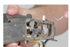
The safety of the K-80 and K-20 can be locked in the "off safe" position and made inoperative. The purpose of this feature is to prevent the loss of a target in competition that results from inadvertently leaving the safety on. This feature is for use ONIY under the controlled conditions
